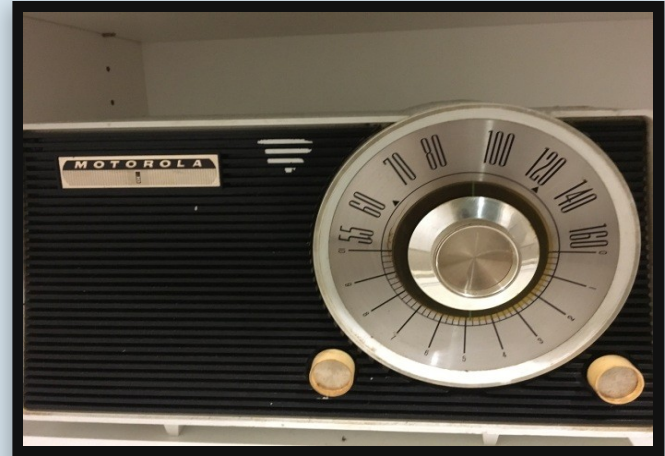
Motorola AM radio showing CONELRAD markers at 640 & 1240 kHz
